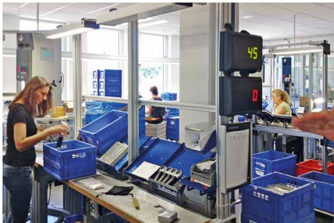
In assembly the quantity of good parts and bad parts is displayed.
